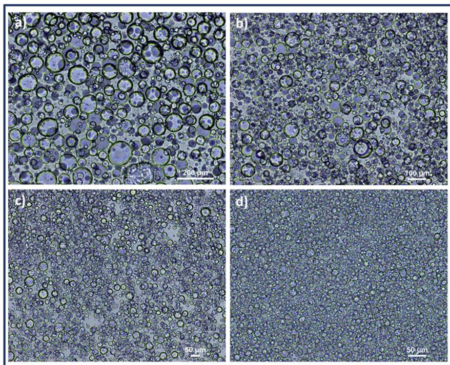
Fig. 2 Light microscope images of PEG-cyclohexanone ( $\phi = 0.25$ ) water in oil silica nanoparticle (1.5%) stabilized Pickering emulsions prepared by vortex times of (a) 30 s, (b) 60 s, (c) 2 min, (d) 8 min.
