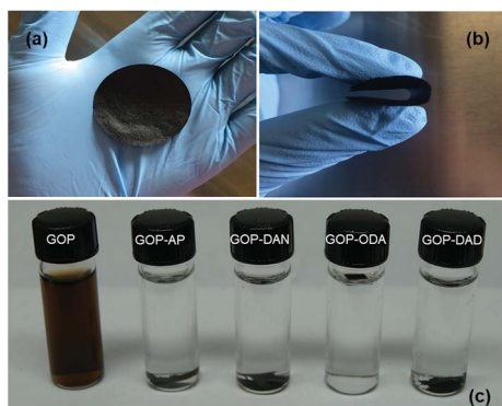
Fig. 2 GOP samples obtained (a) which can be folded without breaking (b). (c) Dispersibility test for pristine and amine-functionalized GOP samples in water after 10 min sonication. After three months, the functionalized samples remained without visible changes.
