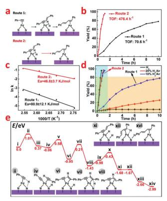
Fig. 4 (a and b) Different routes in the reaction process. (c) Arrhenius plot of the different reaction routes for  $Pd_1/H$ –ZIF. (d) The influence of different atmospheres in different routes. (e) Energies of intermediates and transition states in the mechanism of phenylacetylene dimerization at the  $Pd_1/H$ –ZIF from DFT calculations.
