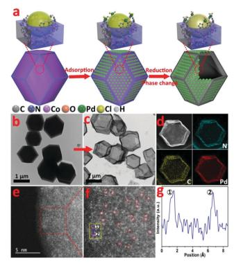
Fig. 1 (a) Schematic illustration of the preparation of Pd<sub>1</sub>/H-ZIF, (b) TEM image of ZIF-67, (c) TEM image of Pd<sub>1</sub>/H-ZIF, (d) corresponding EDS mapping images of N, C and Pd, (e and f) magnified HAADF-STEM images of Pd<sub>1</sub>/H-ZIF, showing that only Pd atoms are present in Pd<sub>1</sub>/H-ZIF, and (g) the corresponding intensity profiles obtained on the yellow area in (f).
