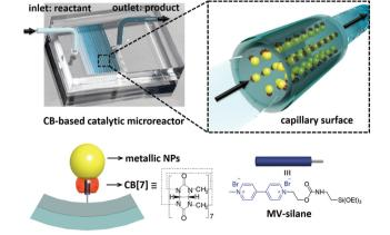
Fig. 1 Schematic illustration of a cucurbit[7]uril-based high-performance catalytic microreactor.
