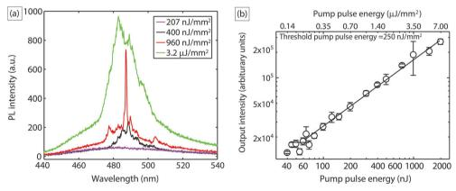
Fig. 5 (a) Spectra obtained from wrapped laser shells at pump energies below and above the lasing threshold. (b) Nonlinear dependence of lasing emission intensity on pump pulse energy. Error bars represent standard deviation obtained from 10 consecutive droplets.
