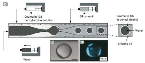
Fig. 4 (a) A schematic of wrapped laser shell generation. (b) Stereomicroscopic image of  $W/O_1/O_2$  droplets and (c) corresponding stereomicroscopic image of  $W/O_1/O_2$  droplets when excited by a pulsed pump laser beam, highlighting WGM light confinement in the shell.
