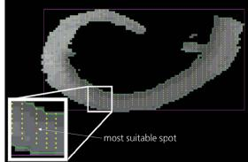
Fig. 4 Left: 3D-detection of object topology exemplarily shown for a cutting; right: processed 3D-image of that cutting with determined bounding box and selected spot suited for LIBS analysis based on geometric criteria, see red spot within enlarged white rectangle. Photos: Fraunhofer II T
