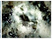
Fig. 5 LIBS measuring spots on an end-of-life refractory brick. Left: refractory brick with three LIBS measuring spots, see white rectangle; bottom, left: broken surface of this material. Middle: enlarged detail corresponding to the white rectangle shown in the left image. Right: detailed view of generated crater with a diameter of about 300 μm. Photos: Fraunhofer ILT.
