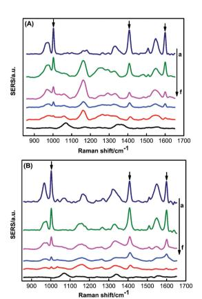
Fig. 6 SERS spectra of triazophos from the surface of cherry tomatoes (A) and plum (B). The concentrations of triazophos were: (a-f) 10  $\mu$ L 50 ppm, 10 ppm, 5 ppm, 1 ppm 0.1 ppm, 0 ppm, respectively. Laser power: 10 mW. Integration time: 50 s. Objective: 20x.
