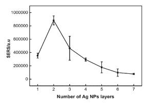
Fig. 3 SERS performance of different Ag NPs rounds-modified PDMS sponge. 10  $\mu$ L R6G (1  $\mu$ M) was used as the Raman probe. Laser power: 14 mW. Integration time: 2 s. Objective: 20x.
