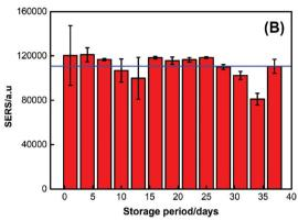
Fig. 4 (A) Statistics of a SERS mapping of a single PDMS sponge-SERS substrate. (B) SERS performance of 20 µL 100 nM R6G on the PDMS sponge-SERS substrate corresponding to different storage periods. The error bar shows the signal variation on a single substrate. Laser power: 10 mW. Integration time: 20 s. Objective: 20x.
