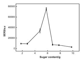
Fig. 2 SERS performance of Ag NPs-modified PDMS sponge prepared with varying amounts of sugar. A total of 10  $\mu$ L of R6G (1  $\mu$ M) was used as the Raman probe. Laser power: 14 mW. Integration time: 2 s. Objective: 20x.
