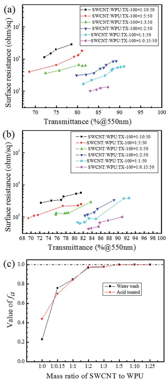
Fig. 3 The relationship between transmittance and sheet resistance of (a) water washed CNT-TAFs and (b) acid treated CNT-TAFs, the points were obtained by changing the dilution of the CNT suspension and wire diameters; (c) adhesion factor ( $f_a$ ) at different mass ratios of SWCNT to WPU.
