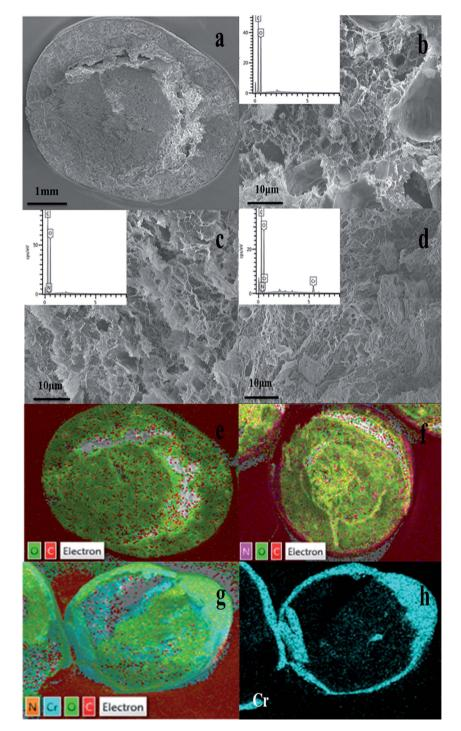
Fig. 8 SEM images of (a, b) CA, (c) CPA-2, (d) CPA-2-Cr; EDX pattern of (e) CA, (f) CPA-2, (g, h) CPA-2-Cr (insets show EDX pattern of element type and content of CA, CPA-2 and CPA-2-Cr).
