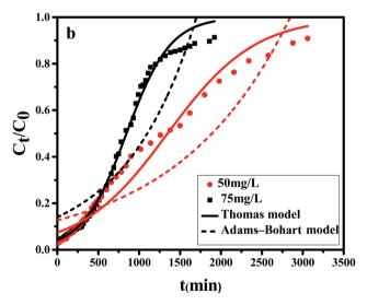
Fig. 7 Experimental and predicted breakthrough curves of Cr(vi) removal by CPA-2 using fixed-bed (a) different flow rates ( $C_0$  = 50 mg L<sup>-1</sup>, H = 8 cm, pH = 2, T = 298 K); (b) different initial Cr(vi) concentrations ( $Q = 1 \text{ mL min}^{-1}$ , H = 8 cm, pH = 2, T = 298 K).
