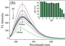
Fig. 5 (a) UV-vis absorption spectra of NCQDs at different pH values. (b) Fluorescence emission spectra of NCQDs at different pH values. Inset shows QYs at different pH values.
