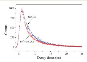
Fig. 8 Fluorescence decay curves of NCQDs in the absence and presence of Fe<sup>3+</sup> ions.
