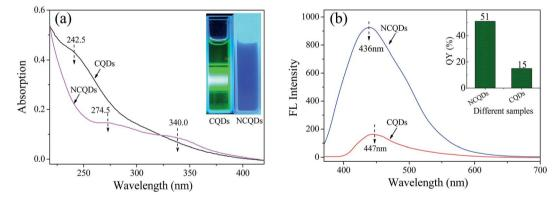
Fig. 4 (a) UV-vis absorption spectra of NCQDs and CQDs. The inset shows digital photographs of CQDs and NCQDs irradiated at 360 nm. (b) Fluorescence emission spectra of NCQDs and CQDs excitated at 360 nm, with  $A_{360}$  < 0.05. The inset shows the QYs of the NCQDs and CQDs.
