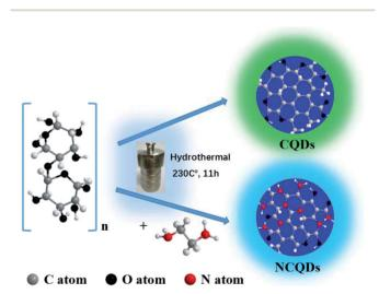
Fig. 1 The synthesis illustration of CQDs and NCQDs.
