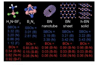
Fig. 11 DDEC6 bonding analysis for five structures containing B-N bonds: H<sub>3</sub>N·BF<sub>3</sub>, B<sub>4</sub>N<sub>4</sub> molecule, BN nanotube, BN sheet, and h-BN solid.
