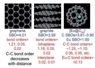
Fig. 10 DDEC6 bonding analysis for three nanostructured materials with a high content of aromatic carbon atoms: graphene, graphite, and  $[Eu@C_{60}]^+$ .
