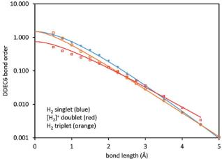
Fig. 4 DDEC6 bond order *versus* stretched bond length for the  $H_2$  singlet,  $H_2$  triplet, and  $[H_2]^+$  doublet spin states. The lines show the fitted model functions listed in Table 2.
