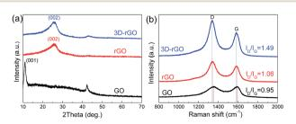
Fig. 2 (a) XRD patterns and (b) Raman spectra of different samples. Here GO, rGO and 3D-rGO denote graphene oxide, reduced graphene oxide and three-dimensional reduced graphene oxide, respectively.  $I_{\rm D}$  and  $I_{\rm G}$  denote the intensities of D-band and G-band.
