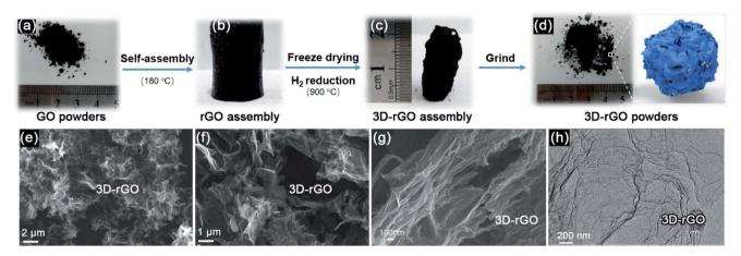
Fig. 1 (a-d) Schematic illustration for the synthesis of three-dimensional reduced graphene oxide (3D-rGO) powders. (e-g) Typical scanning electron microscopy (SEM) images of 3D-rGO powders and (h) transmission electron microscopy (TEM) image of 3D-rGO sample. The right panel of (d) is a schematic structure of 3D-rGO.
