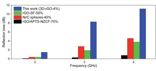
Fig. 5 Reflection loss of different samples in S-band with a coating thickness of 4 mm. rGO–SF with 50 wt% content,  $^{26}$  Ni/C spheres with 40 wt% content,  $^{27}$  rGO/APTS–NZCF with 70 wt% content in matrix.  $^{28}$  Here SF, APTS and NZCF denote hollow glass spheres@Fe<sub>3</sub>O<sub>4</sub>, amino-propyltriethoxy silane and Ni<sub>0.4</sub>Zn<sub>0.4</sub>Co<sub>0.2</sub>Fe<sub>2</sub>O<sub>4</sub>, respectively.
