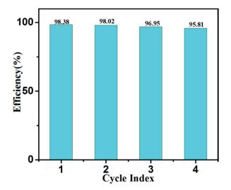
Fig. 8 MB photodegradation activity measured with the recycled catalysts (1–4 cycles, time = 4 h).
