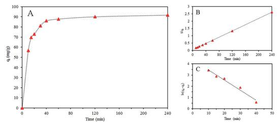
Fig. 7 Effect of time on the adsorption capacity (A), the fitting results of the experimental adsorption kinetic data in terms of pseudo-first-order (B) and pseudo-second-order (C) models (pH: 3,  $Cr(v_i)$  concentration: 100 mg  $g^{-1}$ , volume of  $Cr(v_i)$  solution: 40 mL, adsorbent dose 0.5 g  $L^{-1}$ , and temperature: 298 K).
