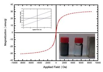
Fig. 4 Hysteresis loop of the SMGO hybrid at room temperature. The top inset: the magnified field from -2 to 2 Oe. The bottom inset: aqueous solution of SMGO (left), separated particles of SMGO by a magnet (right).
