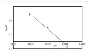
Fig. 11 Plot of  $\ln(q_e/C_e)$  versus 1/T for the adsorption of  $Cr(v_l)$  on SMGO. Mass of SMGO = 0.5 g L<sup>-1</sup>, initial concentration of  $Cr(v_l)$  = 100 mg L<sup>-1</sup>, contact time = 60 min, pH = 3, volume of  $Cr(v_l)$  = 40 mL.
