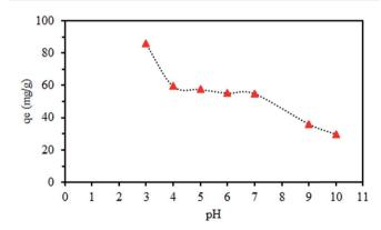
Fig. 6 Influence of initial pH of solution on the adsorption capacity of Cr(vı). Mass of SMGO hybrids = 0.5 g L $^{-1}$ , initial concentration of Cr(vı) = 100 mg L $^{-1}$ , contact time = 60 min, volume of Cr(vı) solution = 40 mL, temperature = 20 °C.
