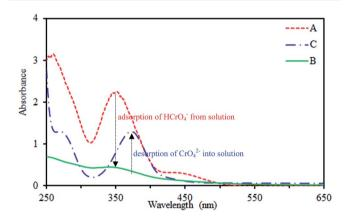
Fig. 9 UV-Vis absorption spectra of the (A) initial solution of  $Cr(v_1)$  (200 mg  $L^{-1}$ ) at pH = 3, (B) adsorption process at T=318 K, and contact time = 60 min (C) desorption process at pH = 10, T=298 K, and contact time = 60 min.
