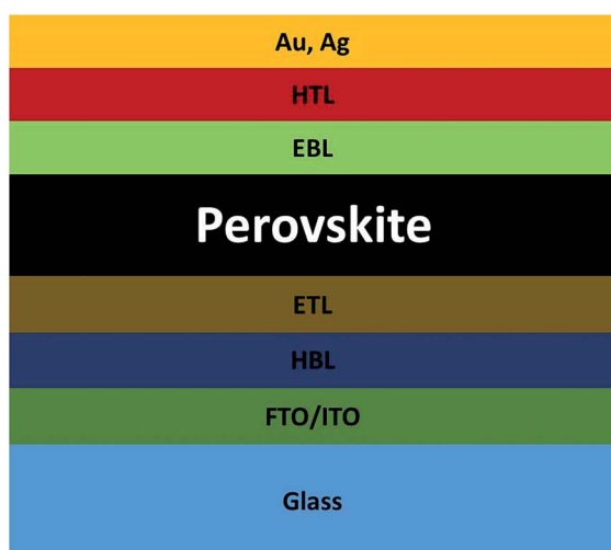
Fig. 1 Schematic of perovskite solar cell.
