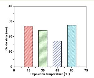
Fig. 10 Effect of deposition temperature on the grain sizes of composite coatings.
