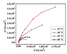
Fig. 13 Effect of deposition temperature on the impedance spectra of composite coatings in 3.5% NaCl solution.
