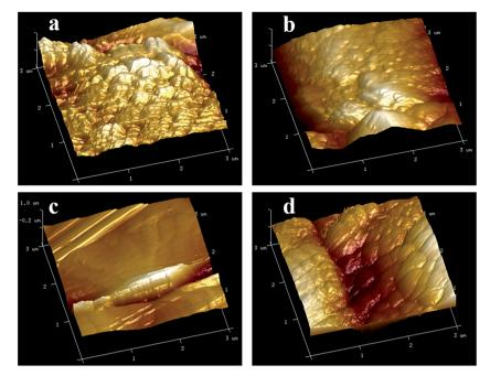
Fig. 5 AFM images (a–d) showing the surface roughness of Ni–graphene composite coatings prepared at deposition temperatures ( $15 \,^{\circ}$ C,  $30 \,^{\circ}$ C,  $45 \,^{\circ}$ C and  $60 \,^{\circ}$ C, respectively).
