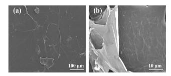
Fig. 1 SEM micrographs of graphene oxide sheets
