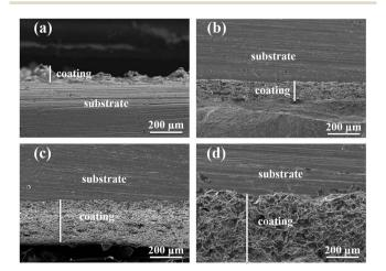
Fig. 7 Cross sectional photographs of the composite coating deposited at different deposition temperatures ((a)  $15 \,^{\circ}$ C, (b)  $30 \,^{\circ}$ C, (c)  $45 \,^{\circ}$ C and (d)  $60 \,^{\circ}$ C).
