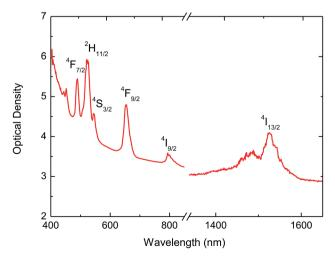
Fig. 5 Absorption spectrum for BaTiO<sub>3</sub>:Er<sup>3+</sup> 9%-Yb<sup>3+</sup> 1% sample.
