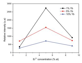
Fig. 7 Relative intensity of up-conversion emission as a function of  $Er^{3+}$  and  $Yb^{3+}$  ion concentrations using  $\lambda_{exc.}=1500$  nm.
