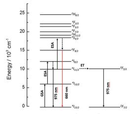
Fig. 11 Energy level diagram for the Er<sup>3+</sup> and Yb<sup>3+</sup> ions, indicating the suggested upconversion mechanisms taking place upon 1500 nm laser excitation.
