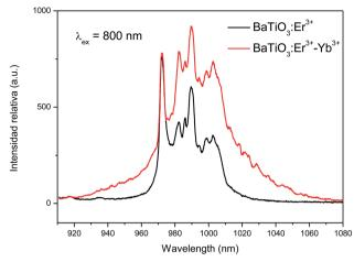
Fig. 10 Emission spectra for BaTiO<sub>3</sub>:Er<sup>3+</sup> 5% and BaTiO<sub>3</sub>:Er<sup>3+</sup> 5%–Yb<sup>3+</sup> 1% exciting at 800 nm.
