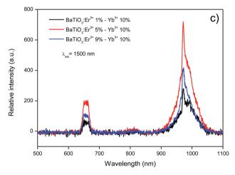
Fig. 6 Up-conversion spectra (excitation at 1500 nm) for BaTiO<sub>3</sub> based phosphors as a function of Er<sup>3+</sup> and Yb<sup>3+</sup> contents
