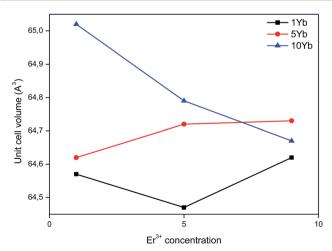
Fig. 2 Variation of the unit-cell volume as a function of the  $\mathrm{Er}^{3+}$  and  $\mathrm{Yb}^{3+}$  contents.
