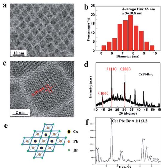
Fig. 2 (a) TEM image of the colloidal CsPbBr<sub>3</sub> NCs. (b) Size distribution analysis for the sample. (c) High-resolution TEM image of the colloidal CsPbBr<sub>3</sub> NCs. (d) XRD patterns of the colloidal CsPbBr<sub>3</sub> NCs. (e) Molecular structure model, and (f) EDX spectrum of the colloidal CsPbBr<sub>3</sub> NCs.
