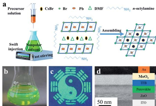
Fig. 1 (a) Schematic of the prepared process for colloidal CsPbBr<sub>3</sub> perovskite NCs, and the precursor solution and assembly into NCs. (b) The optical image of the colloidal nanocrystal solution. (c) The highly luminescent CsPbBr<sub>3</sub> NCs-PMMA polymer patterning, and (d) LEDs using CsPbBr<sub>3</sub> NCs.
