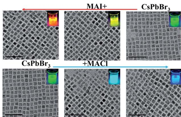
Fig. 4 TEM images of the CsPbBr<sub>3</sub> NCs after treatment with various quantities of MAI (up) and MACl (down). The insets show the evolution of emission colors (under a UV lamp,  $\lambda_{\text{ex}} = 365$  nm) from crude CsPbBr<sub>3</sub> NCs to composited perovskite NCs. Scale bars correspond to 50 nm.
