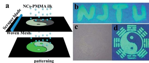
Fig. 6 (a) The schematic of patterning by screen printing. (b), (d) Images ( $\lambda_{\text{ex}} = 365$  nm) and (c) (under daylight) of the patterning obtained using the mixture of CsPbBr<sub>3</sub> NC-PMMA.
