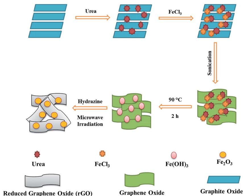
Scheme 1 Schematic of fabrication of rGO-Fe<sub>2</sub>O<sub>3</sub> composite.
