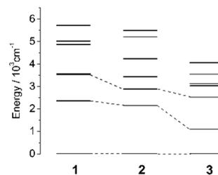
**Fig. 4** Energy level diagram of the splitting of the ground  ${}^4\text{F}$  term for a free  $\text{Co(II)}$  ion in the ligand field of **1**, **2** and **3**. This diagram was extracted from *ab initio* spin-free calculations, and each black line corresponds to a spin-free quartet without SOC. The orbital degeneracy is broken down by the actual geometry, resulting in seven quartets for each complex.
