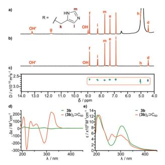
Fig. 4 Spectra of  $(3b)_2 \supset C_{60}$ : (a) <sup>1</sup>H NMR spectrum (600 MHz, CH<sub>3</sub>OH: CD<sub>3</sub>OD, 9:1, v:v), (b) <sup>1</sup>H NMR spectrum with solvent suppression, (c) DOSY spectrum, (d) comparison of the ECD spectra of 3b (green) and  $(3b)_2 \supset C_{60}$  (orange) in MeOH (intensities of ECD spectra were scaled using normalization factors from respective UV spectra), (e) ECD spectra.
