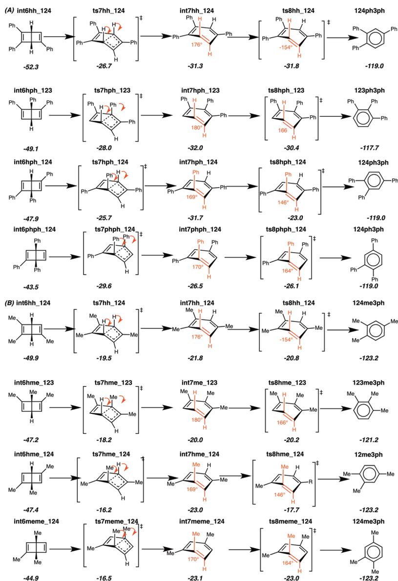
Fig. 8 Structures and free energies, in kcal mol<sup>-1</sup>, for benzene formation from (a) phenyl- and (b) methyl-substituted Dewar benzenes.
