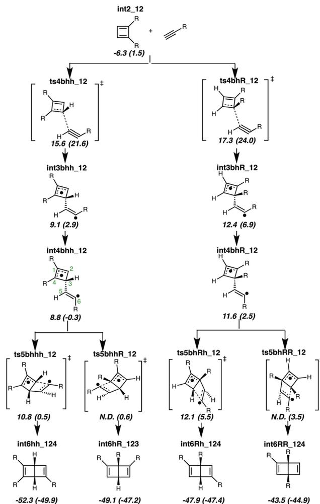
Fig. 4 Structures and free energies, in kcal mol<sup>-1</sup>, for Dewar benzene formation from reactions of substituted cyclobutadienes with phenylacetylene and methylacetylene (in parentheses). [n.d. = not determined].
