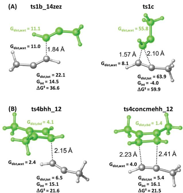
**Fig. 7** Transition structures and free energies, in kcal mol<sup>-1</sup>, for the (a) dimerization of methylacetylene by biradical and carbene mechanisms (b) addition of methylacetylene to 1,2-dimethylcyclobutadiene by biradical and Diels–Alder mechanisms. Distortion energies of the acetylene ( $G_{\text{dist,acet}}$ ), cyclobutadiene ( $G_{\text{dist,cbd}}$ ) and the sum  $G_{\text{dist,tot}}$  are shown, as well as interaction energies ( $G_{\text{tot}}$ ).
