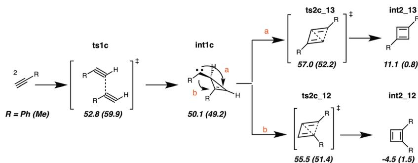
Fig. 2 Structures and free energies, in kcal mol<sup>-1</sup>, for the dimerization of phenylacetylene and methylacetylene (in parentheses) via carbene formation.
