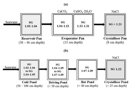
Fig. 3 Schematic illustration of salt production in (a) Goa, India<sup>56</sup> and (b) Maristella salt works at the Western Sicilian Coast.<sup>58</sup> (SG represents the specific gravity calculated from °Bé using the formula SG = 1.45/(1.45 - °Bé)).
