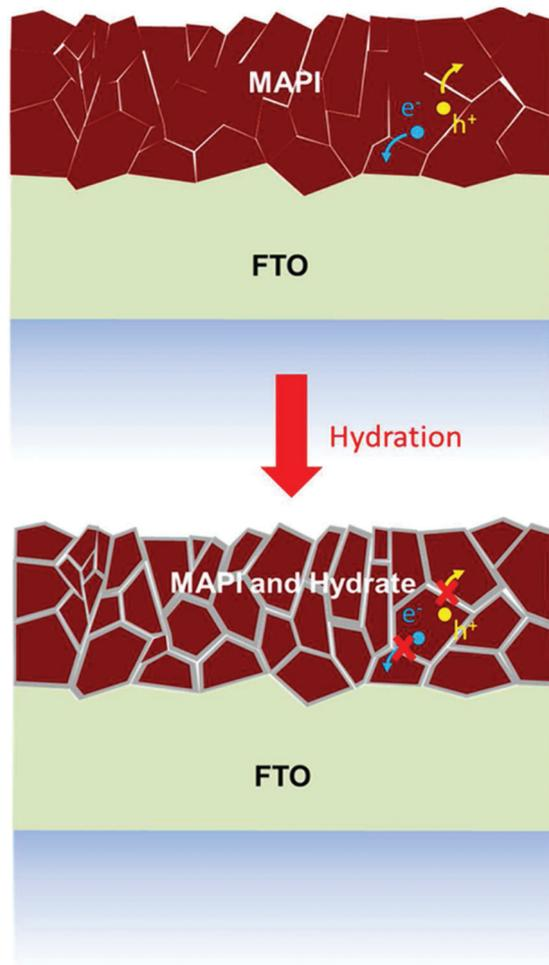
Fig. 11 Microscopic degradation model of MAPbI<sub>3</sub> thin films under partial hydration. Reproduced from ref. 94, Copyright 2015 American Chemical Society.
