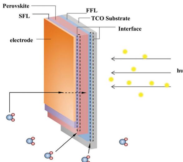
Fig. 14 Two kinds of pathways for intrusion of H<sub>2</sub>O molecules.
