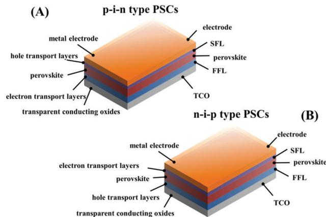
Fig. 1 Schematic of different PSC device architectures.
