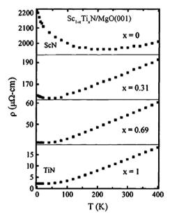
Fig. 1 Electrical properties of ScN, TiN, and ScTiN alloys. From Gall et al.<sup>22</sup> (Copyright American Institute of Physics, used with permission)
