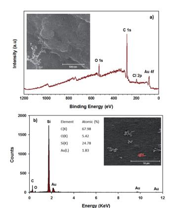
Fig. 3 (a) XPS survey spectra (inset: SEM image of AuNPs-RGO) and (b) EDX analysis (red box in the inset is the selected area for analysis) of RGO-SDBS film after HNO $_3$  and HAuCl $_4$  treatments.
