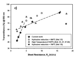
Fig. 4 (a)  $R_{\rm s}$  vs. thickness of the graphene films prepared from four different structures; (b)  $R_{\rm s}$  and transmittance (at  $\lambda=550$  nm) of selected TCGFs with different thicknesses; (c) comparison of  $R_{\rm s}$  as a function of transmittance (at  $\lambda=550$  nm) between our AuNPs–RGO films and other studies. Dash lines show the two regions of differing resistance for the graphene films and the threshold transmittance and corresponding  $R_{\rm s}$ .
