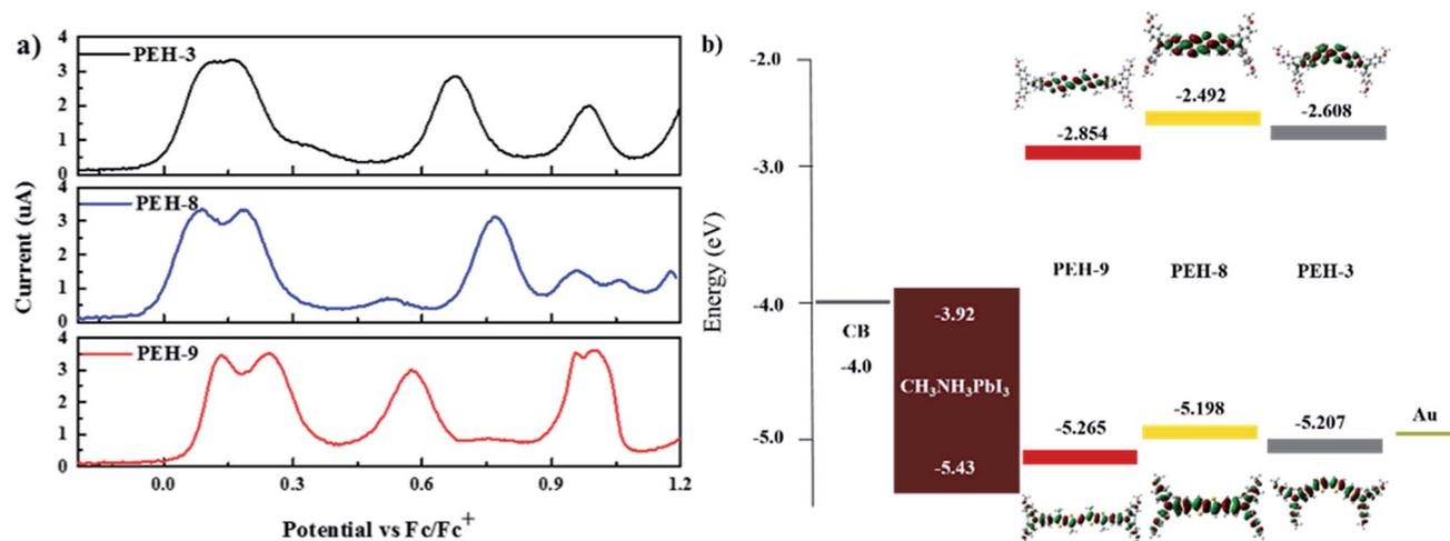
Fig. 3 (a) Differential pulse voltammetry (DPV) of the three compounds with 0.1 M tetrabutylammonium hexafluorophosphate in CH<sub>2</sub>Cl<sub>2</sub> at a scan speed of 50 mV s<sup>-1</sup>, potentials vs. Fc/Fc<sup>+</sup>; (b) energy level diagram of each component in a hybrid solar cell calculated based on DPV measurements with isodensity surface plots of PEH-3, PEH-8 and PEH-9 as calculated by time dependent-density functional theory (TD-DFT) using the B3LYP functional/6-31G\* basis set.
