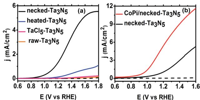
Fig. 2 Current-potential ( $j$ - $E$ ) curves of (a) raw- $\text{Ta}_3\text{N}_5$  (orange),  $\text{TaCl}_5$ - $\text{Ta}_3\text{N}_5$  (pink), heated- $\text{Ta}_3\text{N}_5$  (blue), necked- $\text{Ta}_3\text{N}_5$  (black) and (b) CoPi/necked- $\text{Ta}_3\text{N}_5$  (red) electrode. Electrolyte: 1 M NaOH aqueous solution. Illumination:  $100 \text{ mW cm}^{-2}$ , AM 1.5 G.
