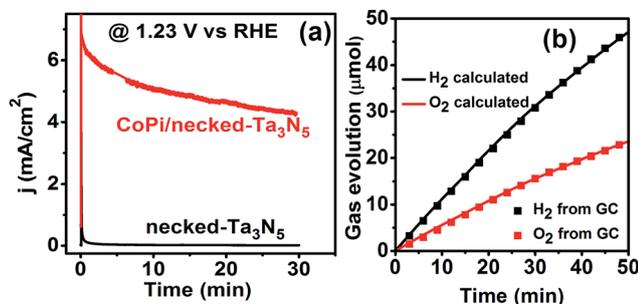
Fig. 7 (a) Stability of the necked-Ta<sub>3</sub>N<sub>5</sub> (black) and CoPi/necked-Ta<sub>3</sub>N<sub>5</sub> (red) photoanodes at 1.23 V vs. RHE. (b) Faradaic efficiency of the CoPi/necked-Ta<sub>3</sub>N<sub>5</sub> photoanode at 1.23 V vs. RHE. Electrolyte: 1 M NaOH aqueous solution. Illumination: 100 mW cm<sup>-2</sup>, Xe lamp (wavelength > 420 nm), area: 0.6 cm<sup>2</sup>.
