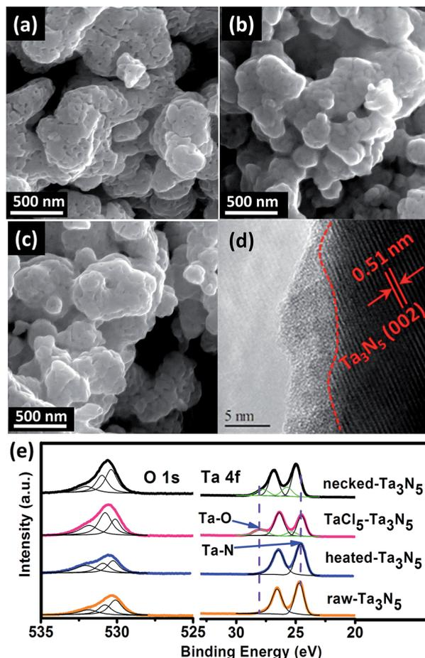
Fig. 1 SEM images of (a) raw-Ta<sub>3</sub>N<sub>5</sub> electrode, (b) TaCl<sub>5</sub>-Ta<sub>3</sub>N<sub>5</sub> electrode, and (c) necked-Ta<sub>3</sub>N<sub>5</sub> electrode. (d) HRTEM image of necked-Ta<sub>3</sub>N<sub>5</sub> electrode. (e) XPS spectra of O 1s and Ta 4f for raw-Ta<sub>3</sub>N<sub>5</sub> (orange), heated-Ta<sub>3</sub>N<sub>5</sub> (blue), TaCl<sub>5</sub>-Ta<sub>3</sub>N<sub>5</sub> (pink) and necked-Ta<sub>3</sub>N<sub>5</sub> (black) electrodes.
