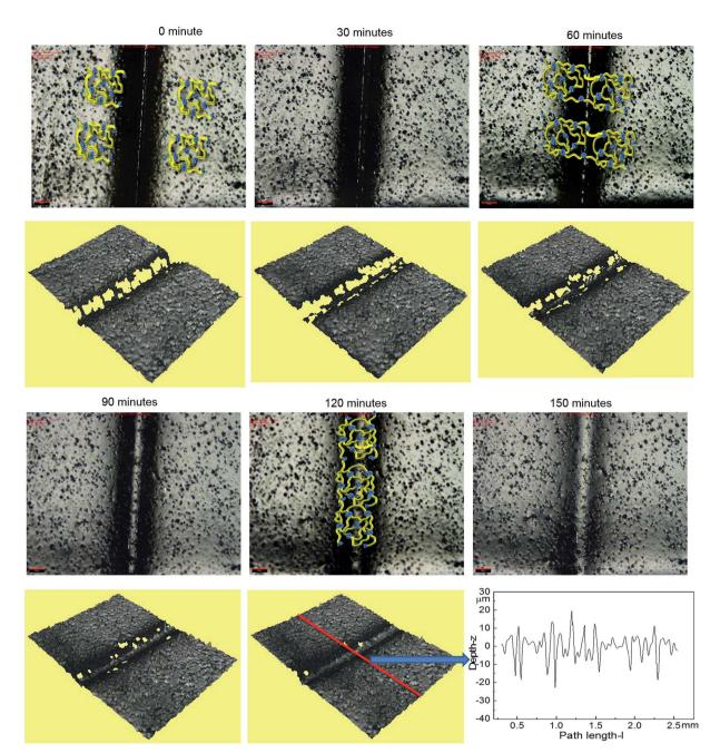
Fig. 4 The dynamics of the healing for polyurethane 1 at the temperature of 37  $^{\circ}$ C (2D and 3D microscopy). The roughness profile is from the middle of the whole sample across the crack horizontally as indicated in the figure by the red line. The scale bar in the picture is 200  $\mu$ m. Cartoons have been added to 0, 60 and 120 minute images to illustrate the healing process.
