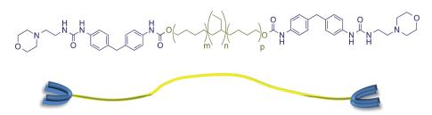
Fig. 1 The supramolecular polyurethane 1 featuring urea morpholine end groups and a schematic representation of this polymer.
