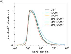
Fig. 2 Performance of the multi-layer OLEDs with various hosts. (a) External quantum efficiency plotted as a function of current density. See Fig. 1a for the device architecture. (b) Electroluminescence spectra at a current density of  $0.1 \, \text{mA cm}^{-2}$ .
