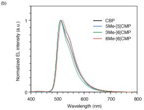
Fig. 5 Performance of the single-layer OLED. (a) External quantum efficiency of the single-layer OLED plotted against the current density. See Fig. 1a for the device architecture. (b) Electroluminescence spectra at a current density of 0.1 mA cm<sup>-2</sup>
