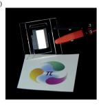
Fig. 9 White OLED with a single-layer architecture. (a) An electroluminescence spectrum at a current density of 0.1 mA cm $^{-2}$ . (b) A picture of the device with an emitting area of 16.6 mm  $\times$  6 mm. The sheet under the device is showing a color reference printed on white paper, and the original colors can be found at http://www.jst.go.jp/erato/isobe/.
