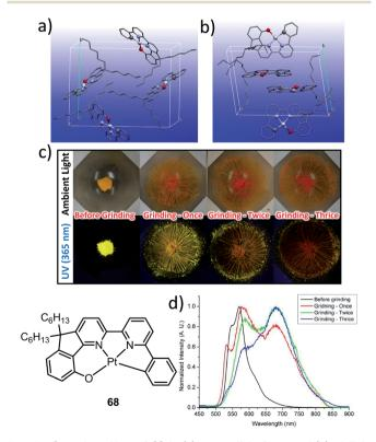
Fig. 12 Crystal packing of 68 in (a) monoclinic form and (b) triclinic form. (c) Photographs of the yellow crystalline solid of 68 before and after grinding under ambient and UV light irradiation (365 nm). (d) Emission spectra of 68 (yellow triclinic form) before and after grinding.
