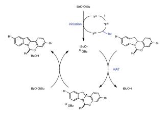
Fig. 6 Proposed chain mechanism.
