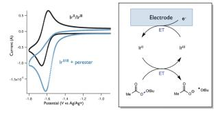
Fig. 12 Voltammetric evidence for catalytic perester reduction by Ir<sup>II</sup>
