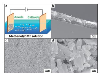
Fig. 2 The schematic diagram of fabrication procedure and SEM images of Zn-MOF/CP cathode using the Zn-MOF synthesized at x = 0.38. (a) Schematic diagram of fabrication procedure. (b) SEM image to show the thickness Zn-MOF on the CP. (c) SEM image of the surface. (d) Amplified SEM image of the surface.
