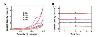
Fig. 6 CV traces (A) and current density profiles at an applied potential of -2.2 V vs. Ag/Ag<sup>+</sup> (B) using different kinds of ILs as electrolytes: (a) BmimBF<sub>4</sub>; (b) BmimOTf; (c) BmimPF<sub>6</sub>; (d) BmimClO<sub>4</sub>.
