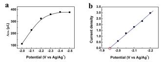
Fig. 5 (a) Amount of  $CH_4$  ( $A_{CH_4}$ , volume at standard temperature and pressure) generated in 2 h under different potentials. (b) Current densities for  $CH_4$  under different potentials and the equilibrium potential can be obtained by extrapolation method.
