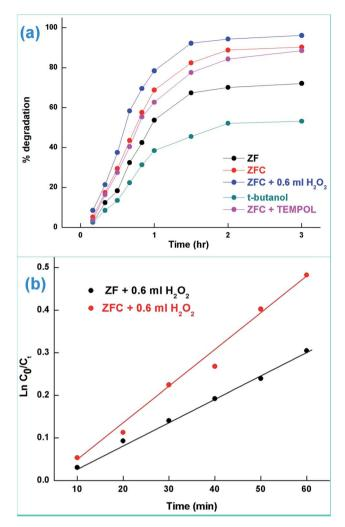
Fig. 8 (a) Degradation of 4-CP under solar light and (b) kinetics plots for 4-CP degradation by ZF and ZFC in the presence of  $\rm H_2O_2$  under solar light (initial pH = 5.5, initial conc. of 4-CP = 20 mg L<sup>-1</sup>, and temperature = 30  $\pm$  0.5 °C).
