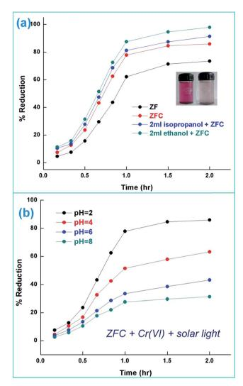
Fig. 7 (a) Photoreduction of Cr(vi) under solar light [initial pH 2],  $Cr(vi) = 70 \text{ mg L}^{-1}$  [temperature =  $30 \pm 0.5 \,^{\circ}$ C] and (b) ZFC performance as photocatalyst with pH variation under solar light.
