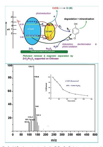
Fig. 9 (a) Band gap structure for the  $ZrO_2-Fe_3O_4$  heterostructure and mechanism of Cr(v) reduction and 4-CP removal and (b) mass spectrum of the solution containing 4-CP after 1 hour of degradation under solar light in the presence of ZFC (inset: COD removal in the presence of ZFC).
