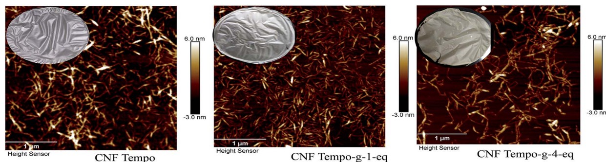
Fig. 5 AFM pictures of CNF Tempo, CNF Tempo-g-1-eq. and CNF Tempo-g-4eq. with films after grafting on the surface of cellulose (conc. 0.1%, tapping mode in air, area 3.3 \times 3.3 \mu\text{m}^2 ).
