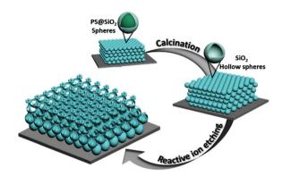
Fig. 1 Schematic illustration of the fabrication process for producing 3D hierarchical nanostructures by direct etching of hollow SiO<sub>2</sub> sphere colloidal crystals via reactive ion etching.
