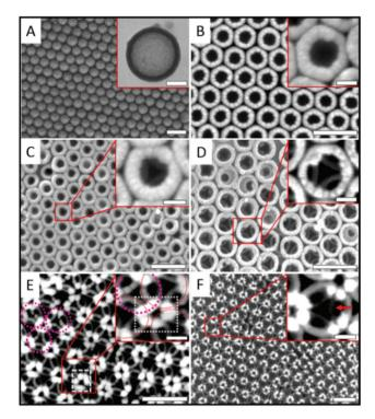
Fig. 2 SEM images show the morphological changes of the hollow sphere colloidal crystals at different etching times: (A) 0, (B) 2, (C) 4, (D) 6, (E) 8, and (F) 9 min. The inset in A shows a TEM image of hollow SiO<sub>2</sub> spheres serving as building blocks in our experiments. The insets in (B-F) are magnified views of the HSCCs. Scale bars: main images, 500 nm; insets in (A-F), 100 nm.
