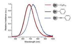
Fig. 3 PL spectra of SiNCs functionalized with n-hexyllithium (red), phenyllithium (black) and lithium phenylacetylide (blue).
