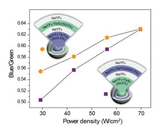
Fig. 7 Power dependent blue-to-green upconversion emission intensity ratio of NaYF<sub>4</sub>:Yb/Tm@NaYF<sub>4</sub>@NaYF<sub>4</sub>:Yb/Er@NaYF<sub>4</sub> and NaYF<sub>4</sub>:Yb/Tm@NaYF<sub>4</sub>@NaYF<sub>4</sub>@NaYF<sub>4</sub>:Yb/Tm@NaYF<sub>4</sub> UCNPs upon 975 nm laser irradiation.
