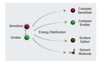
**Fig. 1** Illustration of typical energy distribution processes involving Yb<sup>3+</sup>-sensitized upconversion. Note that for a particular system at the excited state, possible energy distributors include sensitizer ions, codoped emitters, surface defects, and solvent molecules with high energy vibrational groups.
