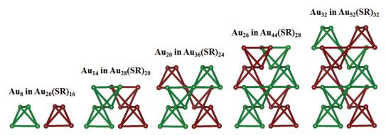
Fig. 2 The structures of  $Au_8$  in  $Au_{20}(SR)_{16}$ ,  $Au_{14}$  in  $Au_{28}(SR)_{20}$ ,  $Au_{20}$  in  $Au_{36}(SR)_{24}$ ,  $Au_{26}$  in  $Au_{44}(SR)_{28}$ , and  $Au_{32}$  in  $Au_{52}(SR)_{32}$ . Au atoms are both olive and wine
