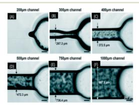
Fig. 11 (A–F) Micrographs of 500  $\mu$ m tall channels built in a range of widths. The actual width of each channels showed deviation of almost 30  $\mu$ m from design. The 300  $\mu$ m wide channel could only be partially cleared of resin, while the smaller channels did not clear at all and larger channels were fully cleared. <sup>60</sup> (Copyright 2015 RSC).
