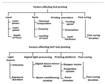
Fig. 8 Parameters affecting laser and DLP-SLA print process.
