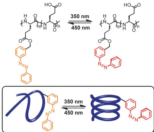
Fig. 2 Poly(L-glutamic acid) containing azobenzene units in the side chains undergoes a photoswitchable coil-helix transition in surfactant-water mixtures leading to turn-on helices.<sup>62</sup>
