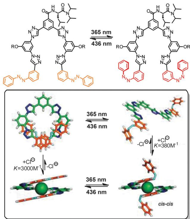
Fig. 10 Photoswitchable clickamer with terminal azobenzene units, which gate the helix-coil transition allowing for light-controlled capture and release of chloride ions.<sup>44</sup>
