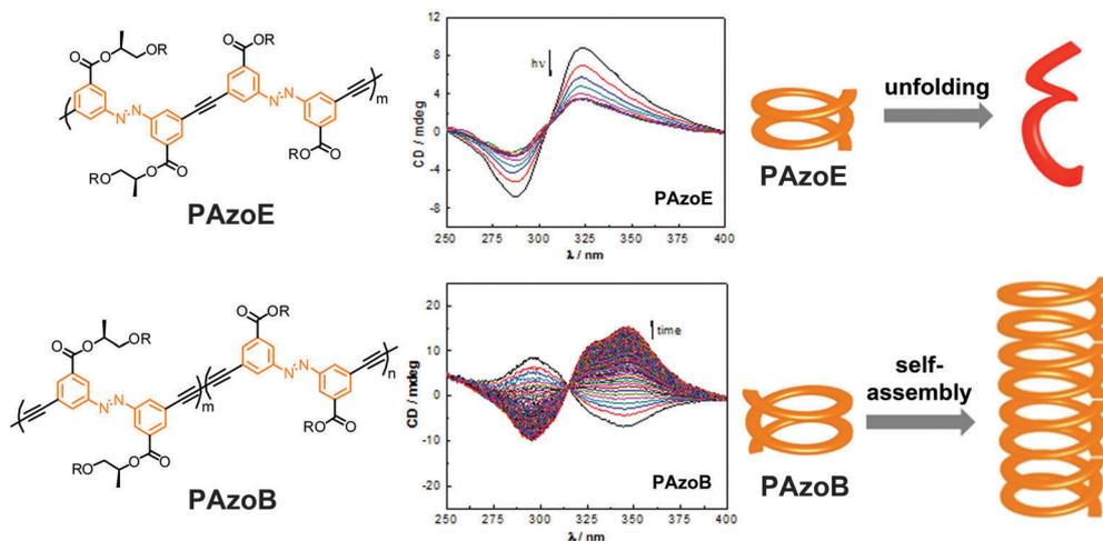
Fig. 20 Polyazobenzene foldamers containing ethynylene (**PAzoE**) and butadiynylene linkages (**PAzoB**) and CD spectra of **PAzoE** upon irradiation ( $\lambda_{\text{irr}} = 358 \text{ nm}$ ) and of **PAzoB** over time in  $\text{CH}_3\text{CN}$  at  $25^\circ\text{C}$ , showing photoinduced unfolding and suppression of photoisomerization due to aggregation, respectively, as illustrated in the cartoon on the right.<sup>109</sup>
