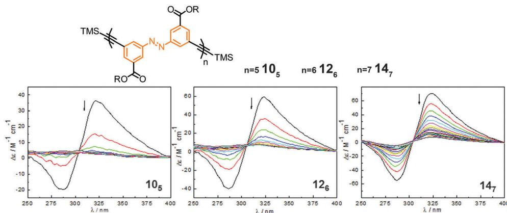
Fig. 14 Photoswitchable oligoazobenzene foldamers **10**<sub>5</sub>, **12**<sub>6</sub>, and **14**<sub>7</sub> (R = -(CH<sub>2</sub>CH<sub>2</sub>O)<sub>3</sub>CH<sub>3</sub> or -(CH(S-CH<sub>3</sub>)CH<sub>2</sub>O)(CH<sub>2</sub>CH<sub>2</sub>O)<sub>3</sub>CH<sub>3</sub>) and their corresponding CD spectra during the course of irradiation at  $\lambda_{\text{irr}} = 358 \text{ nm}$  in CH<sub>3</sub>CN at 25 °C.<sup>45</sup>
