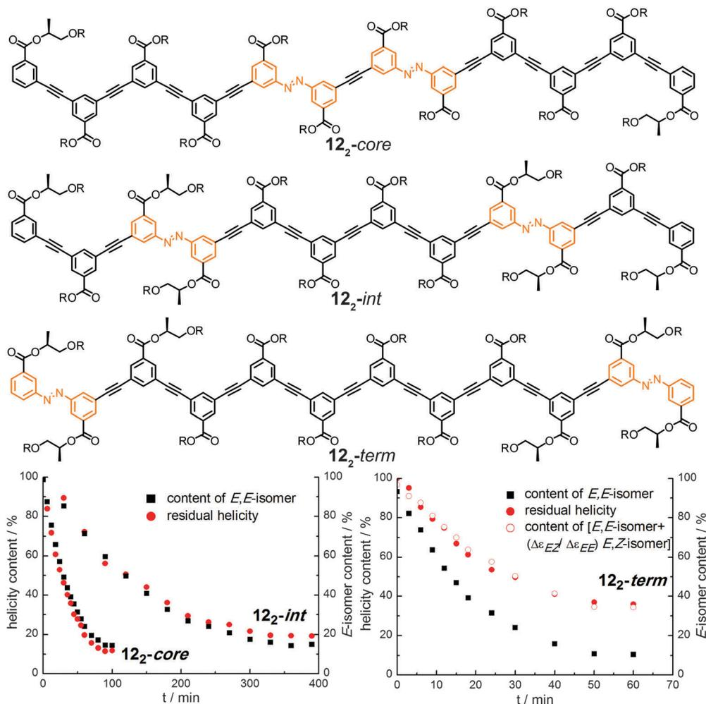
Fig. 17 Photoswitchable oligoazobenzene dodecamers  $12_2$ -core,  $12_2$ -int, and  $12_2$ -term ( $R = -(CH_2CH_2O)_3CH_3$ ) and comparison of their CD intensities and isomer ratios during the course of irradiation at  $\lambda_{irr} = 358$  nm in  $CH_3CN$  at  $25^\circ C$ .<sup>107</sup>
