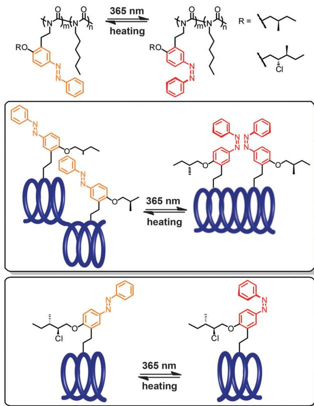
Fig. 5 Polyisocyanates containing chiral azobenzene units (top) exhibiting either a photoswitchable shift in their equilibrium between *P*- and *M*-helical segments (center)<sup>72</sup> or helix inversion (bottom)<sup>73</sup> depending on the number of stereogenic centers in the azobenzene side chain.
