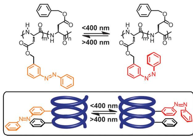
Fig. 3 Poly(L-aspartate) containing *meta*-linked azobenzene units undergoes a photoswitchable helicity inversion (change of helix screw sense) in the mixture of 1,2-dichloroethane and trimethyl phosphate.<sup>64</sup>
