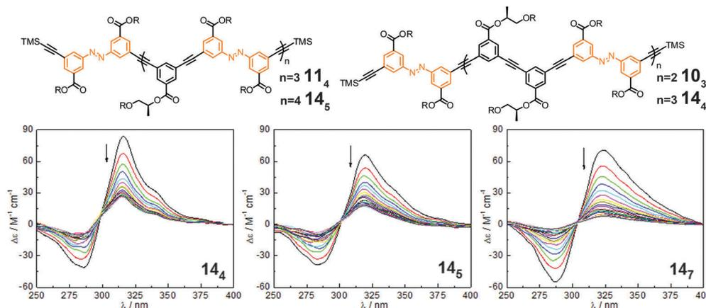
Fig. 15 Photoswitchable oligoazobenzene tetradecamers **14<sub>a</sub>**, **14<sub>b</sub>**, and **14<sub>c</sub>** ( $R = -(\text{CH}_2\text{CH}_2\text{O})_3\text{CH}_3$ ) and their corresponding CD spectra during the course of irradiation at  $\lambda_{\text{irr}} = 358$  nm in  $\text{CH}_3\text{CN}$  at  $25^\circ\text{C}$ .<sup>106</sup>
