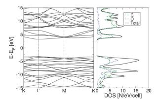
**Fig. 2** Electronic band structure of fully oxidized graphene (left) and total density of states (right), calculated using the PBEO exchange correlation functional.
