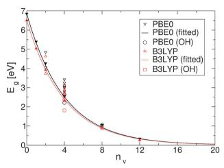
Fig. 4 Dependence of the fundamental energy gap as a function of the number of O vacancies,  $n_v$ . For  $n_v = 2$  and  $n_v = 4$  energy gaps for all possible configurations are depicted. Solid lines are fits through the calculated values for most stable structures. Circles and squares represent structures with added hydroxyl groups.
