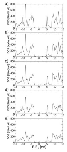
Fig. 6 Evolution of the total density of states of rGO with: (a) one O vacancy, (b) two O vacancies, (c) four O vacancies, (d) eight O vacancies, and (e) twelve O vacancies, for most stable structures inside each configuration. All total DOS were calculated using the PBEO exchange correlation functional.
