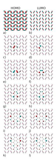
Fig. 7 Highest occupied (HOMO) and lowest unoccupied (LUMO) molecular orbitals: (a and b) fully oxidized graphene, (c and d) one O vacancy, (e and f) two O vacancies, (g and h) four O vacancies, (i and j) eight O vacancies, and (k and l) 12 O vacancies. Red and blue denote opposite signs of the wavefunction.
