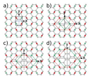
Fig. 9 Symmetries of several representative unit cell structures: (a) fully oxidized graphene surface,  $C_2^{\nu}$ , (b) single O vacancy,  $C_2^{\nu}$ , (c) two vacancies,  $C_2^{\nu}$ , and (d) four O vacancies,  $C_2^{\nu}$ . All arrangements in unit cells with  $n_{\nu} \neq 0$  corresponding to those with minimal energy.
