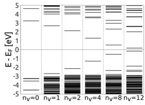
Evolution of the electronic structure change and the energy gap with the increase of the number of O vacancies,  $n_v$ . On the left side the electronic states at the  $\Gamma$  point of the fully oxidized graphene are also presented. All results are obtained by the PBEO exchange correlation functional.
