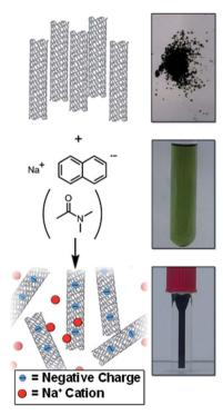
Fig. 1 Schematic (left) and pictures (right) of raw SWCNT powder and NaNp solution in DMAc forming a solution of nanotubide.
