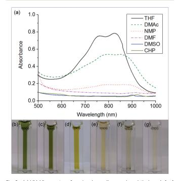
Fig. 2 (a) UV-Vis spectra of equimolar sodium and naphthalene (of  $\sim$ 1 mg<sub>(Na)</sub> mL<sup>-1</sup>) added to a selection of solvents. (b–g) Cuvettes containing the Na + Np solutions of (b) THF (c) DMAc (d) DMF (e) NMP (f) DMSO (g) CHP.
