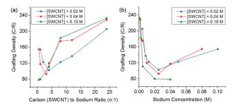
Fig. 5 Grafting density of reduced SWCNTs added to 1-bromododecane versus (a) C: Na ratio, (b) sodium concentration, illustrating a shifting ideal stoichiometry but a stable sodium concentration.
