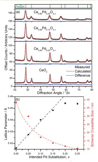
Fig. 2 (a) Fits to powder XRD data ( $\lambda = 1.54056$  Å) of  $Ce_{1-x}Pd_xO_{2-\delta}$ (x = 0, 0.05, 0.10, 0.20). Tick marks above denote positions of fluorite cell, space group  $Fm\bar{3}m$ . (b) Refined lattice parameter, a, and crystallite size as a function of intended Pd substitution, x. In (b) the linear fit of lattice parameters is over the range  $0 \le x \le 0.15$  (see text for discussion) and the curved line is a guide to the eye.
