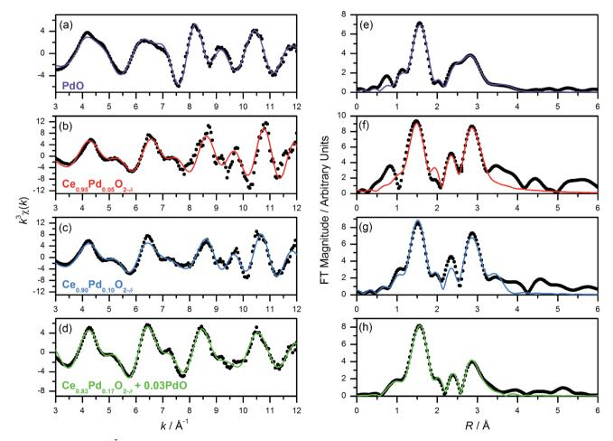
Fig. 4 (a-d) Pd K-edge  $k^3$ -weighted EXAFS spectra (points) with fits (lines); and (e-h) Fourier transforms of PdO,  $Ce_{0.95}Pd_{0.05}O_{2-\delta}$ ,  $Ce_{0.90}-Pd_{0.10}O_{2-\delta}$  and  $Ce_{0.80}Pd_{0.20}O_{2-\delta}$  (nominal composition), respectively.
