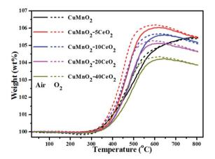
Fig. 4 TGA curves of the as-prepared CuMnO<sub>2</sub>-xCeO<sub>2</sub> samples (i.e., post-annealed at 960 °C under flowing Ar for 12 h) under flowing air or pure  $O_2$  with 25 mL min<sup>-1</sup> from room temperature to 800 °C. The solid lines are the TGA curves under air and the short dashed lines are the TGA curves under pure O<sub>2</sub>
