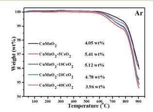
Fig. 7 TGA curves of oxidized CuMnO<sub>2</sub>–xCeO<sub>2</sub> samples (*i.e.*, after the TGA test up to 800 °C under flowing O<sub>2</sub>) from room temperature to 900 °C under flowing argon with 25 mL min<sup>-1</sup>.
