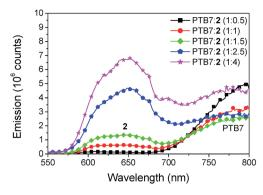
Fig. 9 Fluorescence emission spectra of PTB7: 2 for varying blend ratio. The excitation wavelength was 280 nm. The emission at 650 originates from compound 2 and the emission at 800 nm from PTB7.
