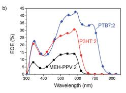
Fig. 4 EQE spectra of MEH-PPV (squares), P3HT (circles) and PTB7 (diamonds) blended with compound 1 (a) and compound 2 (b).
