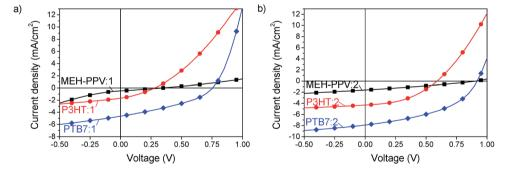
Fig. 5 JV-characteristics of acceptors 1 (a) and 2 (b) blended with MEH-PPV (squares), P3HT (circles) and PTB7 (diamonds).
