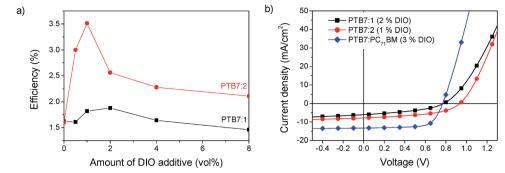
Fig. 7 (a) Power conversion efficiency of PTB7:1 and PTB7:2 as a function of the amount of solvent additive DIO. (b) JV-curves of optimized solar cells in comparison to PTB7:PC<sub>71</sub>BM
