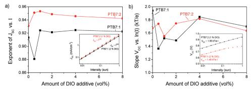
Fig. 8 (a) The exponent of the short circuit density vs. light intensity (I) as a function of content of DIO. The inset shows an example at the optimized conditions. (b) Slope of the open circuit voltage as a function of content of DIO. The inset shows an example at the optimized conditions.
