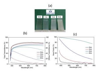
Fig. 1 (a) Optical appearance, (b) UV-Vis total and diffuse transmittance and (c) haze factor spectra of ZnO films prepared with various acetic-acid contents in precursor solutions.
