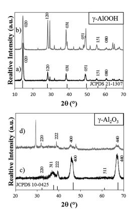
Fig. 5 Assigned X-ray diffraction pattern for  $\gamma$ -AlOOH (a) nanorods and (b) nanoplates synthesised under acidic and basic conditions respectively (200 °C, 20 h) and  $\gamma$ -Al<sub>2</sub>O<sub>3</sub> (c) nanorods and (d) nanoplates. (Acidic = pH 3.5, basic = pH 12.8).
