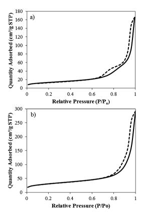
Fig. 6 Nitrogen adsorption—desorption isotherms at  $-196\,^{\circ}\text{C}$  of (a)  $\gamma$ -AlOOH synthesised at 200  $^{\circ}\text{C}$  for 20 h with 1 M NaOH and (b) corresponding  $\gamma$ -Al $_2$ O $_3$  after calcination. (Adsorption = solid line, desorption = dashed line).
