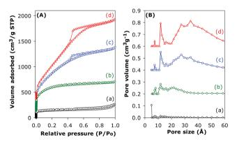
Fig. 8 Nitrogen sorption isotherms (A) and pore size distribution curves (B) of (a) pristine (CNT-as) sample and activated CN4T samples; (b) CN4600, (c) CN4700 and (d) CN4800.
