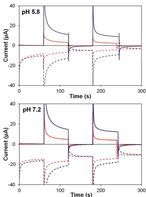
Fig. 6 Photoelectrochemical generator-collector measurements (chronoamperometry) of TiO<sub>2</sub>-P2 (red) and TiO<sub>2</sub>-2 (dark blue) at pH 5.8 and pH 7.2. Solid lines are the photoanode current; dashed lines, collector current; collector efficiency ca. 60%. Applied bias 0 mV vs. Ag/AgCl, illuminated with a 455 nm LED (33 mW cm<sup>-2</sup>). Photocurrent densities are reported in Table 4.
