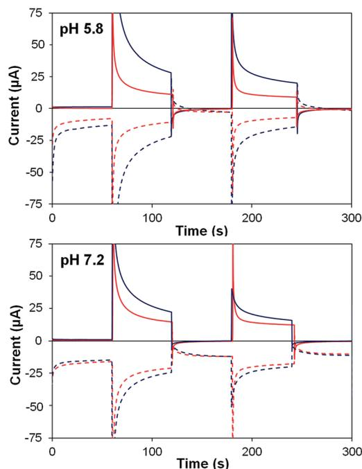
Fig. 7 Photoelectrochemical generator–collector measurements (chronoamperometry) of  $\text{TiO}_2\text{-2}$  (red) and  $\text{TiO}_2\text{-2Na}_2\text{-1}$  (dark blue) at pH 5.8 and pH 7.2. Solid lines are the photoanode current; dashed lines, collector current; collector efficiency *ca.* 60%. Applied bias 0 mV vs.  $\text{Ag}/\text{AgCl}$ , illuminated with a 455 nm LED ( $33 \text{ mW cm}^{-2}$ ). Photocurrent densities are reported in Table 4.
