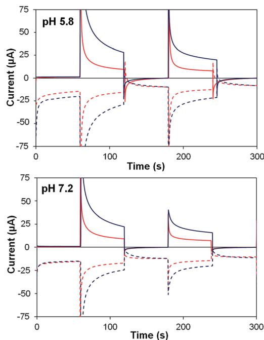
Fig. 8 Photoelectrochemical generator–collector measurements (chronoamperometry) of  $\text{TiO}_2\text{-P2-1}$  (red) and  $\text{TiO}_2\text{-2Na}_2\text{-1}$  (dark blue) at pH 5.8 and pH 7.2. Solid lines, photoanode current; dashed lines, collector current; collector efficiency *ca.* 60%. Applied bias 0 mV vs.  $\text{Ag}/\text{AgCl}$ , illuminated with a 455 nm LED ( $33 \text{ mW cm}^{-2}$ ). Photocurrent densities are reported in Table 5.
