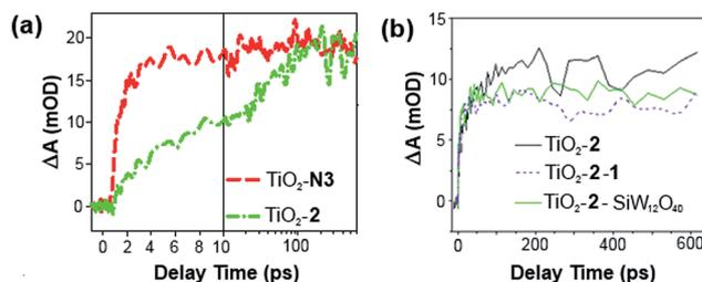
Fig. 4 Mid-IR comparison of the kinetics of electron injection in (a) TiO<sub>2</sub>-**2** and TiO<sub>2</sub>-N3, and; (b) TiO<sub>2</sub>-**2**-**1** and TiO<sub>2</sub>-**2**-SiW<sub>12</sub>O<sub>40</sub>. Data have been scaled to the absorbance of the supporting dyad film.
